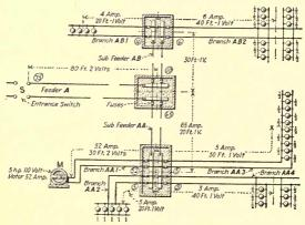
Fig. 94.—Wire sizes for an installation.
